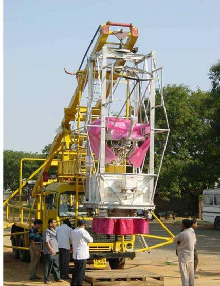
**Figure 5.** T100 cm IR telescope instrument on the launch truck.
