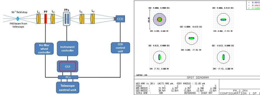
**Figure 2.** Left: Schematic of a dual FP based narrow band imager. Right: Diffraction limited spot diagram of the optical design.
