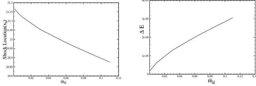
**Figure 1.** *Left panel:* Variation of shock location with disk accretion rate, which decreases with increasing disk rate for the fixed halo rate 0.5. *Right panel:* Variation of the cooling energy with accretion rate, which also implies that the increase in disk rate increases the amount of cooling of the post-shock region.
