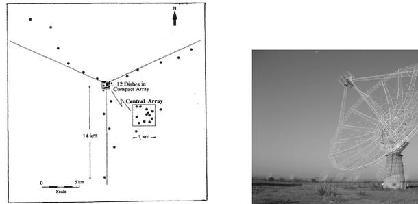
**Figure 9.** GMRT consists of 30 parabolic dishes of 45 m diameter each and are located in a Y-shaped array of 25 km in extent.
