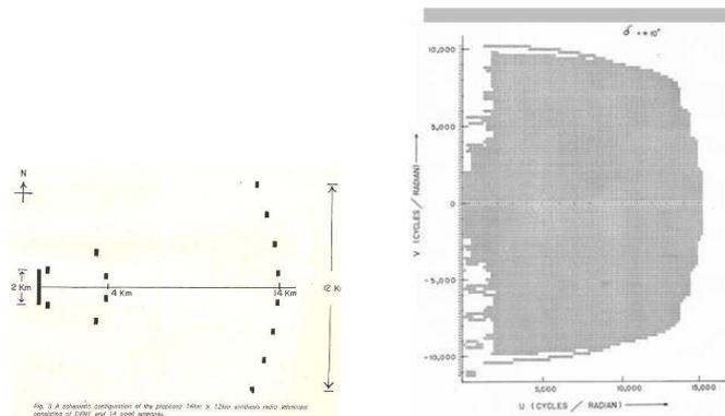
**Figure 8.** Arrangement of the proposed Giant Equatorial Radio Telescope (GERT) in 1979, to be constructed at the Earth's equator (left) and its UV diagram (right). GERT consisted of a 2 km long and 50m wide NS parabolic cylindrical antenna and fourteen 100m long and 50m wide parabolic cylindrical antennas placed upto 14km away.
