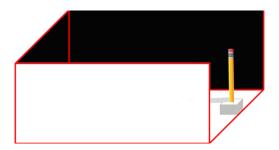
Take a box of approximate size 30 cm x 30 cm x 30 cm. Cut off the top and one side. Stick good, white, non-shiny paper at the base of the box. Paint the other three sides with dull matt black paint or line them with rough black paper. At one end stick a bar of thermocol or some material into which you can mount a vertical object like a pencil. Place the unit such that the open side faces Venus. Watch carefully. You should be able to see a faint but distinct shadow of the pencil.
