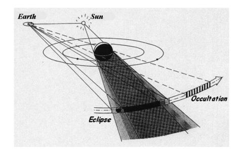
Eclipses occur when the satellites pass in the shadow of Jupiter. Occultations occur when the satellites pass behind Jupiter for a terrestrial observer
